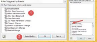
• It is then necessary to set an Event Trigger for the checking rule in your templates, "After Save Document" is a good choice for this. To set the Event Trigger, go to the Manage tab of Inventor, the iLogic panel and select Event Triggers. This will display a dialog where the user selects the event, then the Select Rules button. This will display another box where the user can select the rules to be run on that event.
