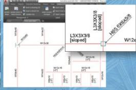
Use snap points to efficiently dimension anchors on drawings
